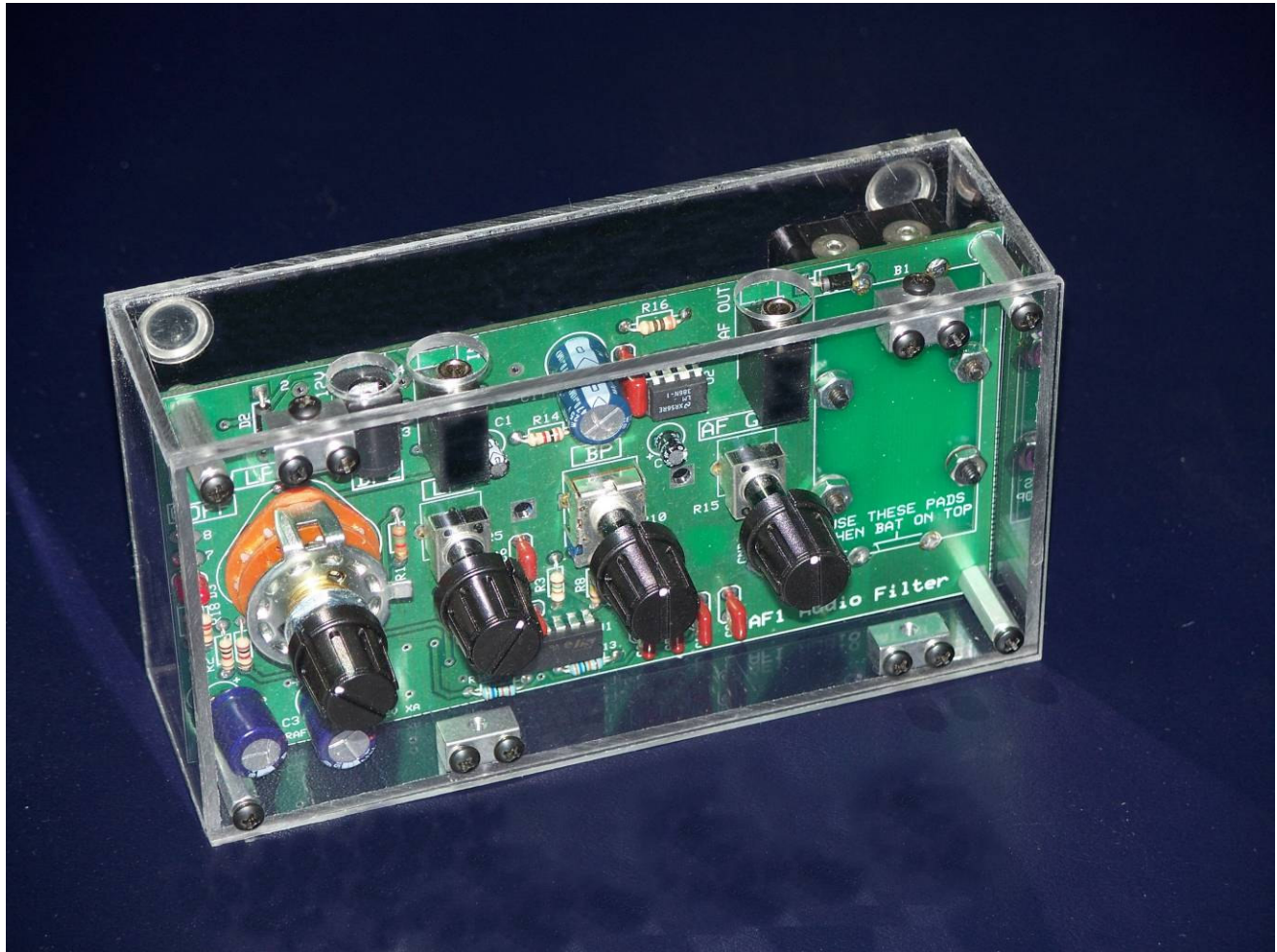
Elecraft AF1 Audio Filter Mounted in the AF1 Enclosure
