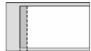
Score and remove 1/8" of the cover from tape
